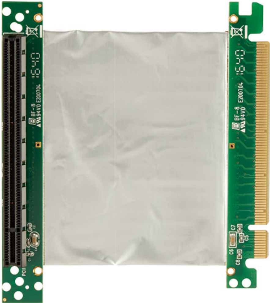
PClex16 to PClex16 riser card, L=100 mm
